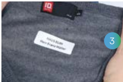
(3) Corrected result: Thanks to the thin, elastic and soft material, the new label lies perfectly flat — the incorrect heat-sealing is no longer visible.
