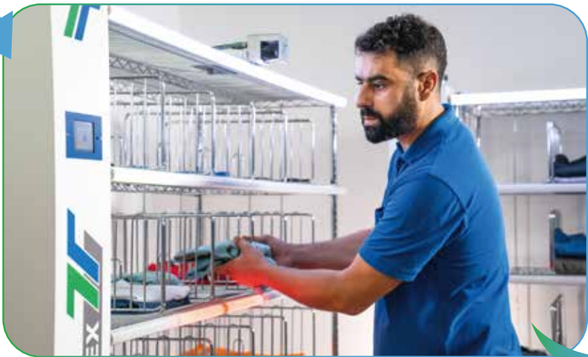
Step 3: A red light signal clearly indicates the wrong compartment and reliably prevents incorrect allocation. The green signal confirms the correct compartment — the laundry has been sorted correctly and the process is completed properly.
