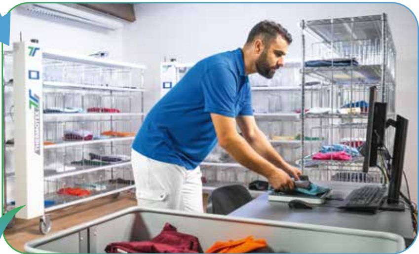
Step 2: Using barcode, Data Matrix, or RFID identification, each garment is uniquely assigned and prepared for sorting.
